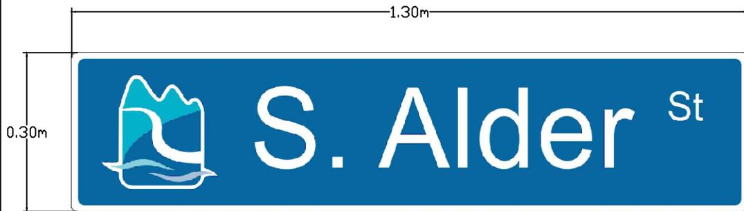
SIGNALIZED INTERSECTION STREET SIGN FACE SHALL BE NON-REFLECTIVE COLOURED BACKGROUND WITH DIAMOND GRADE REFLECTORIZED WHITE CHARACTERS, BOTH SIDES.
