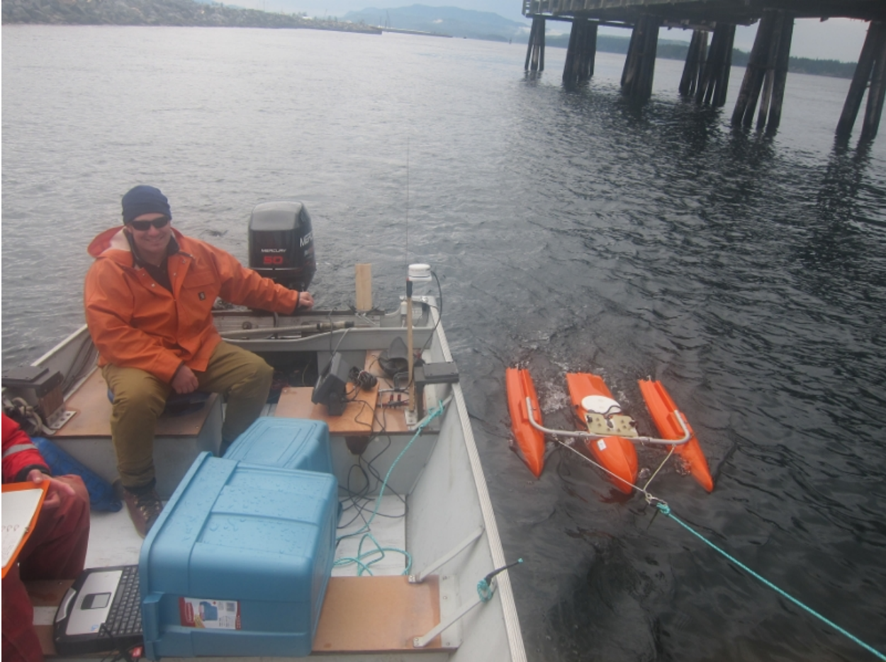
Figure 4.4: Photo of Ecofish Research technicians taking current measurements inside the Campbell River Fishing Pier. The orange catamaran is the Teledyne River Ray ADCP which is being towed from the boat using a boom. Ecofish staff Ian Murphy is piloting the boat and Andrew Cline (obscured to left) is monitoring the measurements.
