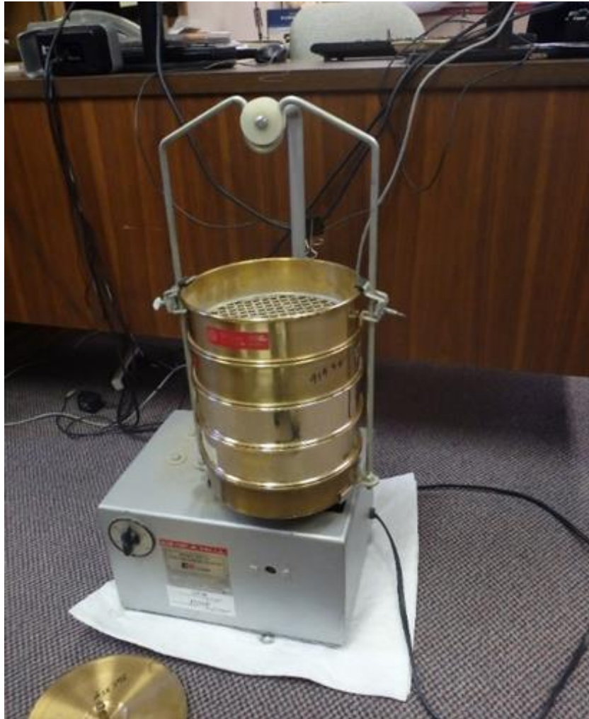
PHOTO 12: STACK OF SIEVES (9.5 MM, 1.0 MM, 0.42 MM AND 0.21 MM) AND SHAKER MACHINE USED FOR THE GRAIN SIZE ANALYSIS.
