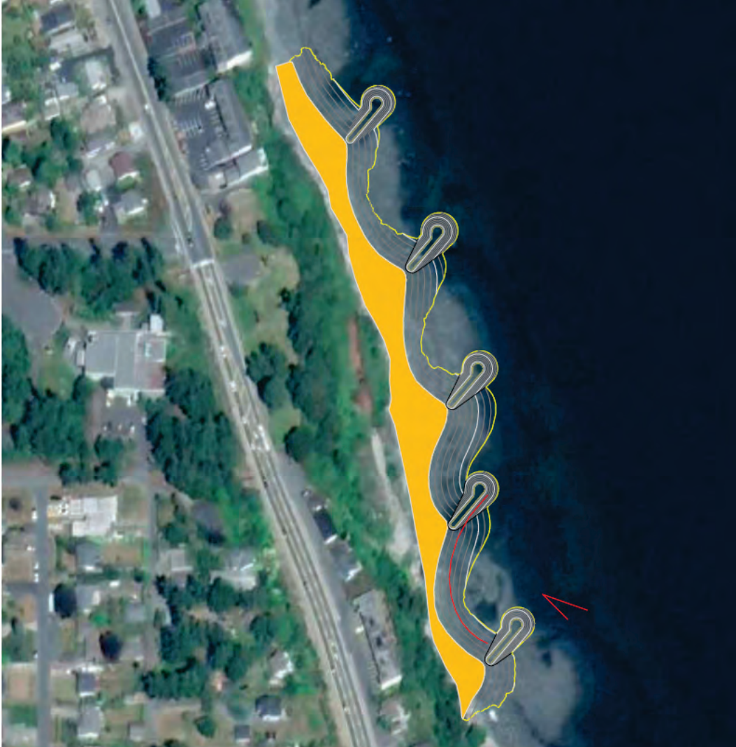
Figure 4-19: Sketch of a Pocket Beach system at Sequoia Park beach. Beach shape and headland spacing designed using the equilibrium embayment methodology. Red arrow shows the incident wave direction for the pocket beach shape.
