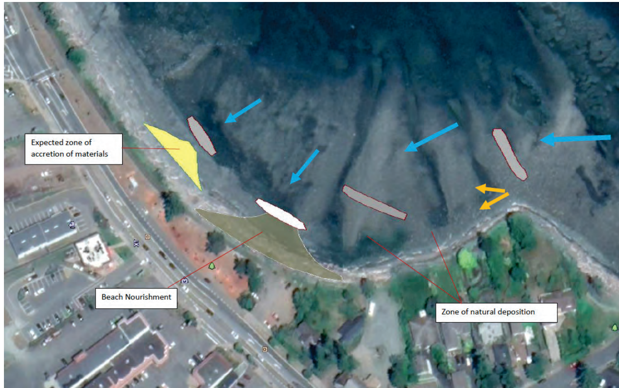
Figure 4-26: Plan of potential pocket beach and offshore headland mitigation for Frank James Park, as modeled with SWASH. Blue arrows show principal wave directions and orange arrows show area of expected wave diffraction. Four rock armour structures are shown. Grey structures have crest elevations of 3.5 m while the white shaded structure has a crest elevation of 2.8 m. A recommended area of a beach nourishment is shown in tan, while the yellow zone indicates an area where natural accretion is expected.
