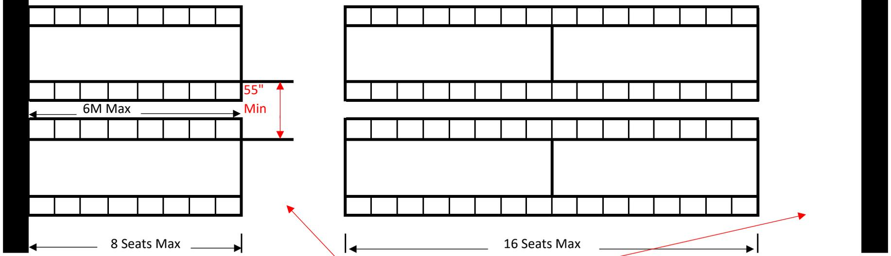
Aisle width to be a minimum 44 " except for aisles serving rows where there are 60 seats or fewer must be a minimum 30 " wide
