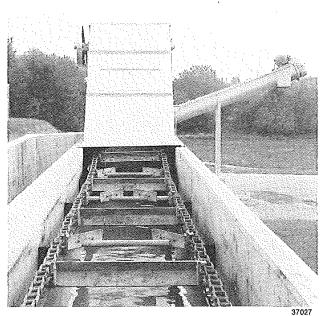
Type B Straightline grit collectors. Type SW grit washer dewaters and washes the grit prior to discharge to ground or truck.
