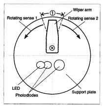
① Rest position of the wiper arm Tolerance range: ±20°
