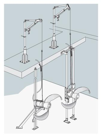
**Single guide bar system** A frequently used solution that eliminates any risk of fatigue, yet provides a cost efficient installation. **Double guide bar system** Rigid design that also allows installation of multiple mixers at different depths.
