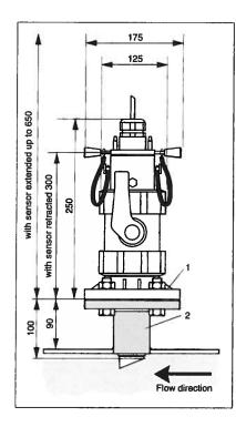
Dimensions of Probfit CUA 461 assembly 1 Process connection DIN Flange DN 50 or ANSI 2\* 2 Process connection adapter
