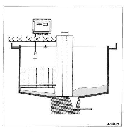
Continuous separation level measurement in sludge thickener
