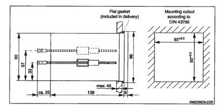
Installation of panelmounted housing
