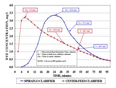
plug flow relationship for a centerfeed clarifier. Although not related to this project, the CH2M-Hill study showed that the Spiraflo Clarifier design was as effective hydraulically as a 40-to-1 length to width ratio typical chlorine contact tank design.
