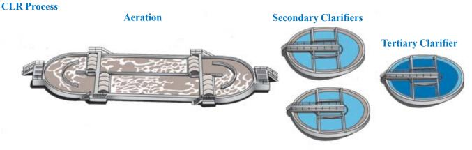
This diagram illustrates a typical series clarification operation.
