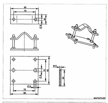
Post mounting kit for installation of field housing on cylindrical pipes (horizontal or vertical, max. Ø 60 mm; see Accessories)
