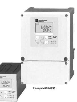
Due to the modularity of its design, the Liquisys M CUM 223 / 253 transmitter can be adapted to a wide range of customer needs. The basic version. which provides simple measuring and alarm signalling functions, can be equipped with additional software and hardware modules to match specific applications. Retrofitting of expansion modules is also possible.
