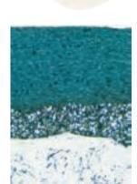
Cross section of Flygt epoxy coating
