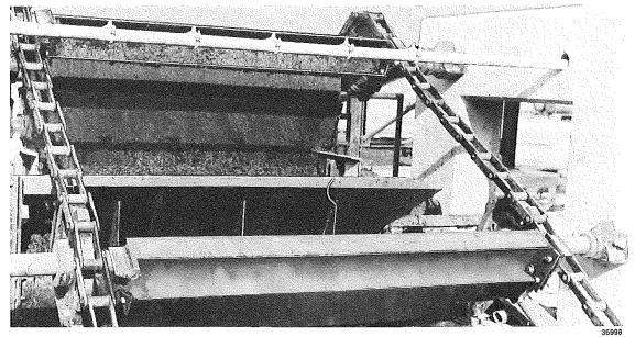
Type B chain and bucket collector removing bark from a pulpwood flume settling basin.
