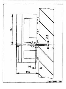
Wall mounting Screws: Ø 6 mm Anchors: Ø 8 mm
