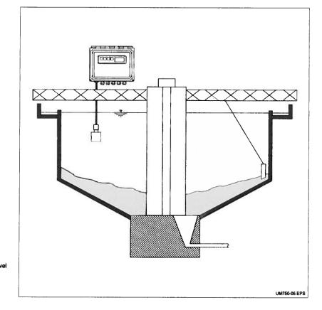
Continuous sludge level measurement in primary clarifier. Installation on scraper bridge
