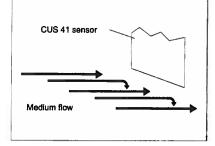
Self-cleaning by flow against the inclined
