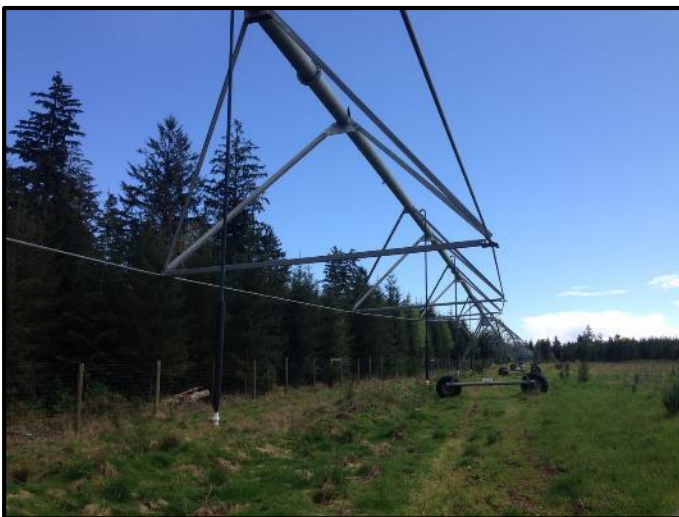
Photograph 3: An irrigation pivot used to land-apply liquid biosolids from the Norm Wood Environmental Centre. (April, 2015)
