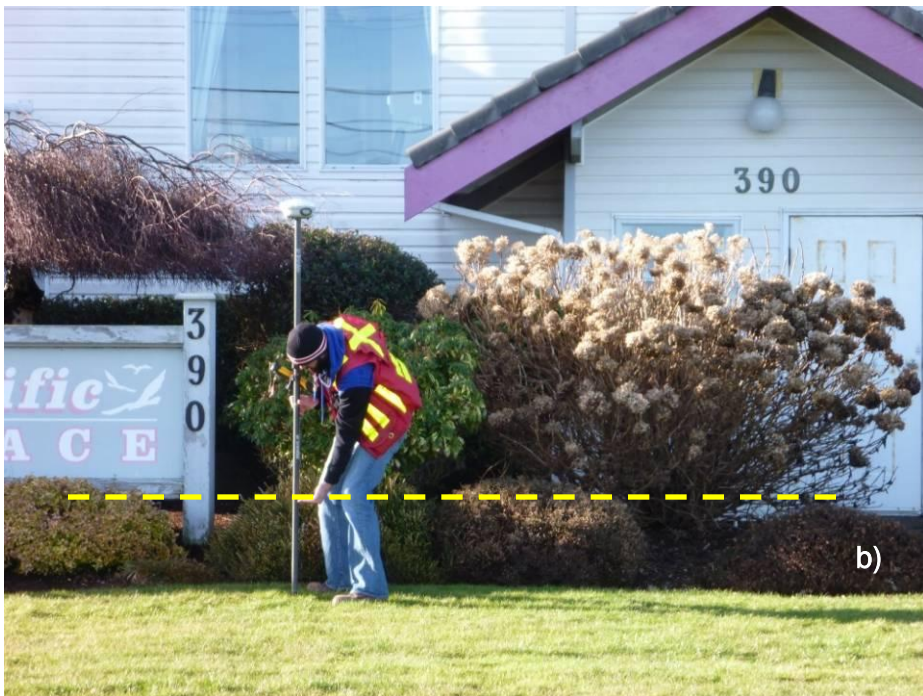
Figure 8. Surveyor indicating the elevation of the draft BC Flood Construction Level (with proposed sea level rise included at a) Ocean Grove, and b) near Rotary Beach Park (photos taken 17 January 2011).
