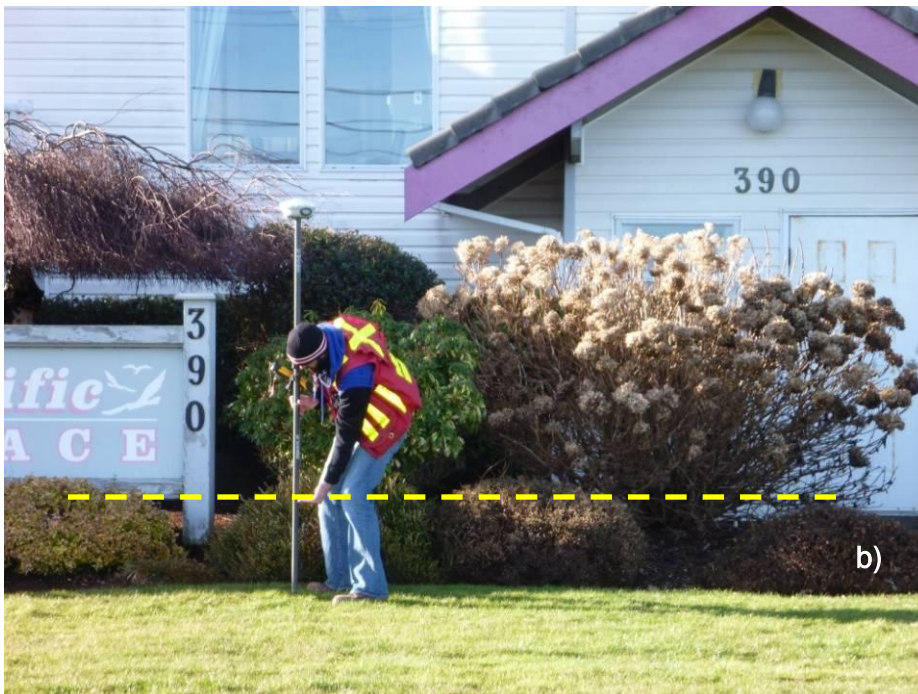
Figure A-28. Surveyor indicating the elevation of the draft BC Flood Construction Level (with proposed sea level rise included at a) Ocean Grove, and b) near Rotary Beach Park (photos taken 17 January 2011).
