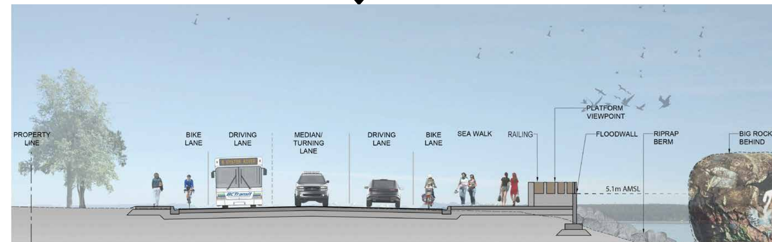
Sea "Wall" Section: Near the Big Rock, a floodwall will be constructed to protect the road and walkway. A viewing platform is proposed to be integrated.
