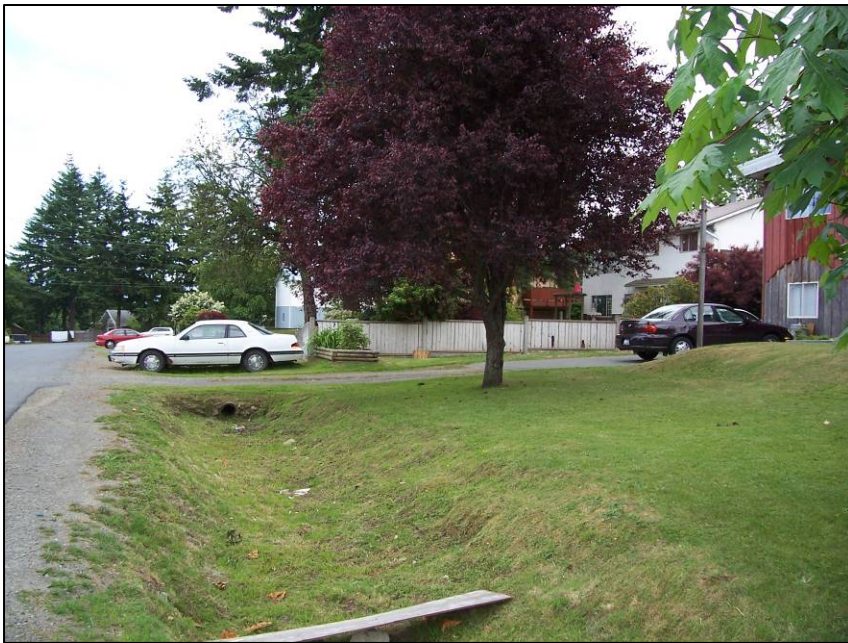
Typical residential streets in upper Campbellton Area; note ditch which could be converted to a bioswale for runoff treatment
