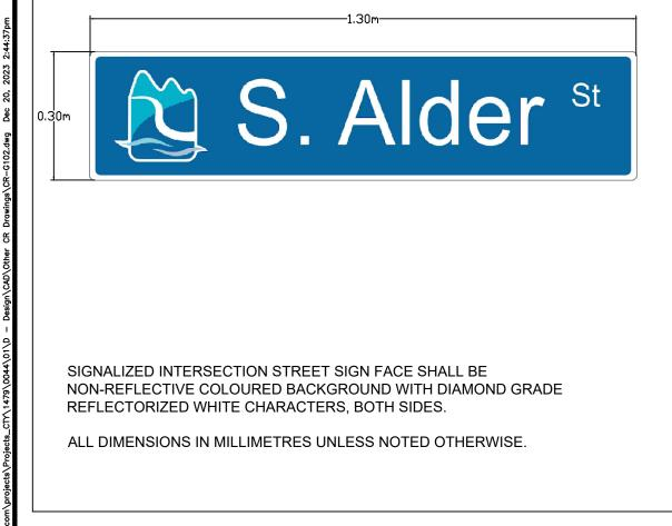
SIGNALIZED INTERSECTION STREET SIGN FACE SHALL BE NON-REFLECTIVE COLOURED BACKGROUND WITH DIAMOND GRADE REFLECTORIZED WHITE CHARACTERS, BOTH SIDES.
