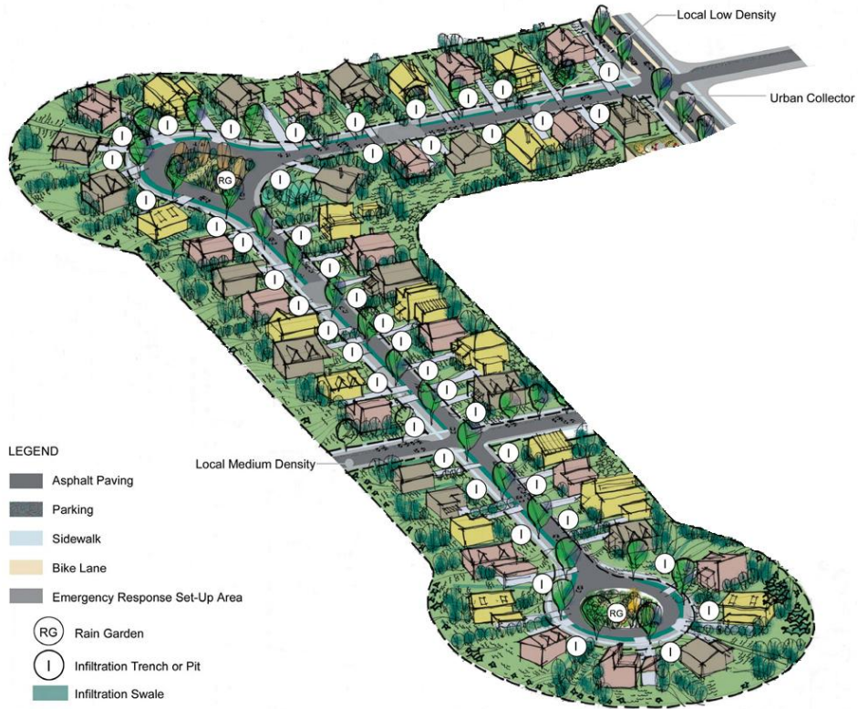
Figure 4-1 – Potential Integration of Stormwater Source Controls into Residential Development
